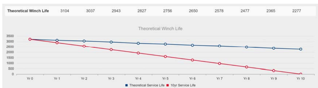
Figure 4 CICA Winch Life Calculation
